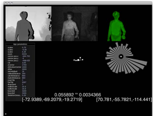
Fig. 2: Combined view of game visuals and debug information. On top (from left to right): depth image, greyscale image and user silhouette. In the middle: the player skeleton (from above). On the right: a sound item with spectral visualization.
